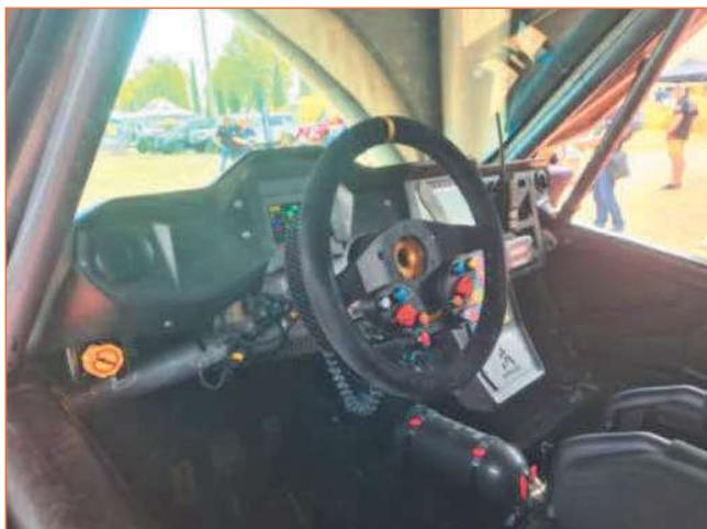
Fig. 3: Equipped dashboard integrating recycled carbon mat © VESO Concept
