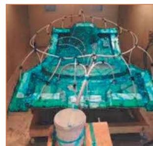
Fig. 2: Roof panel under vacuum © VESO Concept
